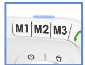
Answer the calls from the Voice base and call the 3 direct memories, even if the handset is not on the cradle
